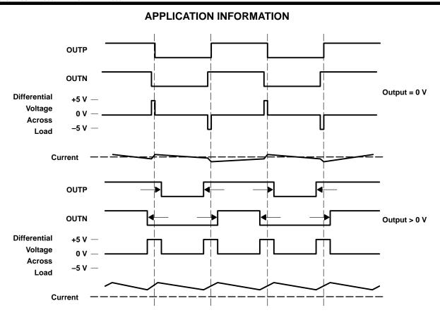
Figure 11. The TPA2000D1 Output Voltage and Current Waveforms Into an Inductive Load
