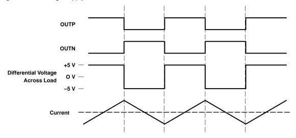
Figure 10. Traditional Class-D Modulation Scheme Output Voltage and Current Waveforms Into an Inductive Load With No Input
