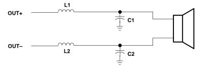
Figure 1. Class-D Output Filter
