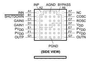
NC – No internal connection, still requires a pad for the ball.NOTE: The shaded terminals are used for thermal connections to the ground plane.
